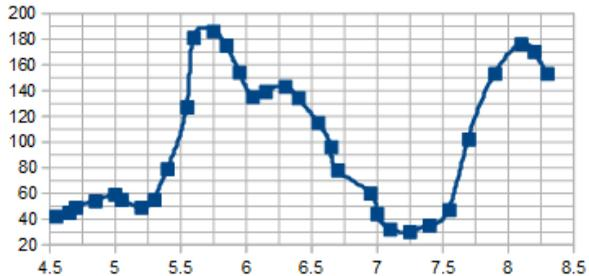
Output from Teraterm user interface above: First peak of power level 190 at 5.6MHz (does not light receiver LEDs). Second peak level 180 at 8.1MHz illuminates receiver's LEDs. Interesting the ratio of these two frequencies is not 2.0 as predicted by conventional wisdom, rather it is 8.1MHz/5.6MHz=1.4. Hence longitudinal wave is the second maximum, and transverse wave is the first maximum. Transverse wave decreased strength at a distance, longitudinal did not.
