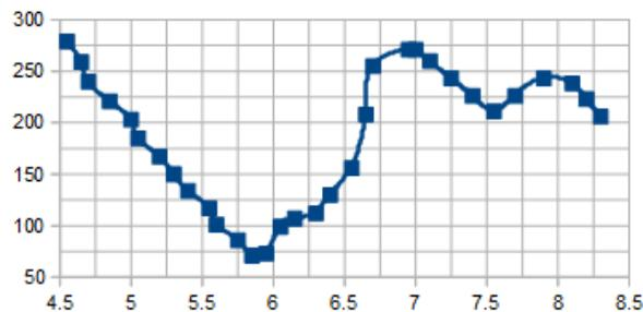
Output from Teraterm user interface above: In near field (42 inches transmitter to receiver), the receiver LED remains illuminated above 6MHz.
